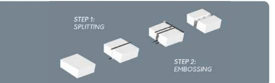
**Innovative in every detail - Calsitec-Combi-Embosser** is a combined splitting and embossing unit that performs two processing steps in one machine run. In one punching process one brick is split and at the same time two brick halves are embossed to produce a stretcher and a header at the same time.
