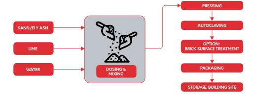
Every raw material is stored separately. According to the production recipe sand/fly ash and lime are weighted in weighing containers and forwarded to the mixer. Here the raw materials are mixed to a homogeneous mixture in short time. According to the sand moisture and the recipe some water can be added to the mixture. One mixing cycle lasts for ca. 3 minutes.
