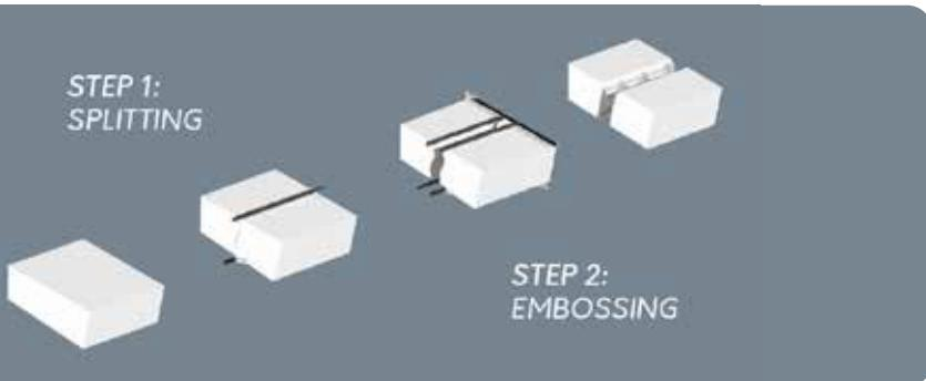
**Innovative in every detail - Calsitec-Combi-Embosser** is a combined splitting and embossing unit that performs two processing steps in one machine run. In one punching process one brick is split and at the same time two brick halves are embossed to produce a stretcher and a header at the same time.
