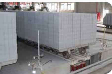
Once the bricks have been pressed, they are automatically removed from the press with a gripper, placed on a hardening trolley and forwarded to autoclaves with a traverser that can transport up to 6 hardening trolleys. The traverser picks up loaded hardening trolleys from the press, forwards them to the autoclaving area and loads the autoclaves.
