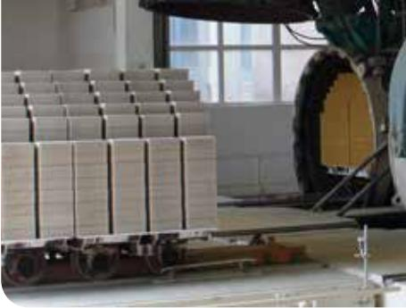
During this time the brick structure is changing. The mass made of lime, sand and water begins to interact and to form a robust structure of the CSU. During hardening process the silicic acid on the grain surface of silica sand is loosened under the influence of hot water vapour atmosphere. The silicic acid together with a binder – lime hydrate – form crystalline phases (CSH phases), that grow on sand grains and strongly bind them together.
