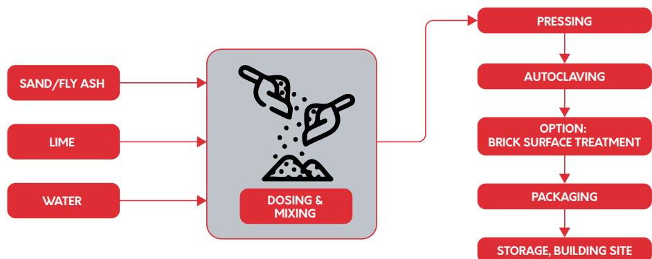
Every raw material is stored separately. According to the production recipe sand/fly ash and lime are weighted in weighing containers and forwarded to the mixer. Here the raw materials are mixed to a homogeneous mixture in short time. According to the sand moisture and the recipe some water can be added to the mixture. One mixing cycle lasts for ca. 3 minutes.
